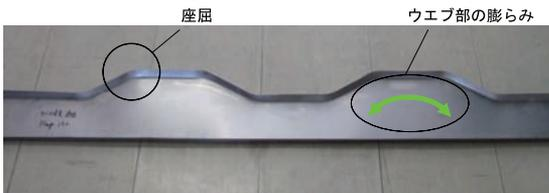
Fig.5 A sample of flexible channel section
