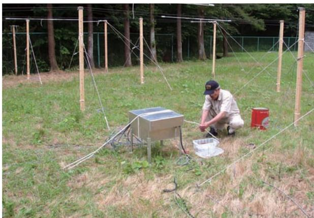
Fig.7B Imaging riometer receiver box in the center of antenna area
